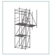
**Step 8:** Continue to add and push out steel planks along ledger to fill cantilevered bay.
