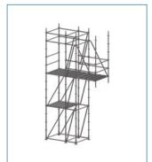
**Step 12:** Scaffolder walks out to end of cantilevered bay behind advanced guardrail and installs guardrail and mid rail at outer standards.
