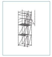
**Step 4:** Remove tie and push pre-assembled cantilever/spur needle to the outside of the scaffold.
