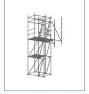
**Step 7:** From behind the guardrail, place steel plank on the cantilevered ledgers.
