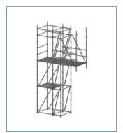
**Step 11:** Install intermediate putlog as the advanced guardrail solution and remove guardrails on end of main scaffold structure.
