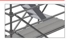
**Lift-off locks:** These components, which lock planks against wind lift off, are very important in high wind or cyclone risk areas where the risk of component dislodgement is increased.
