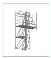
**Step 10:** Hammer home pins in ledger connections to the rosette.
