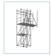
**Step 9:** Install guardrail and midrail to cantilevered bay from behind guardrail of main scaffold.
