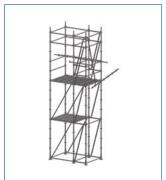
**Step 3:** Connect diagonal brace to the utmost rosette of the main scaffold structure.
