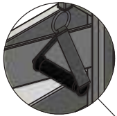
STIRRUP HANDLE TO RELEASE HEIGHT LOCKING PINS IN 280MM INCREMENTS
