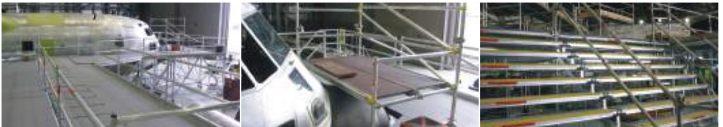
MOBILE SCAFFOLDING FOR WING PROTECTION DESIGNED TO AVOID USING HARNESSES AND LANYARDS
