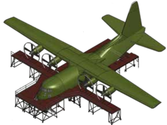
MOBILE ALUMINIUM DOCKING FOR NOSE AND PROPELLER ACCESS UNIQUE SLIDING PLATFORM SYSTEM FOR CLOSE ACCESS TO FUSELAGE
