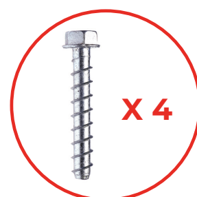
10 x 100mmL concrete screw anchor *90mm embedment
