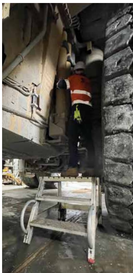
Handles for manoeuvrability, simply lift to engage the front wheels.
