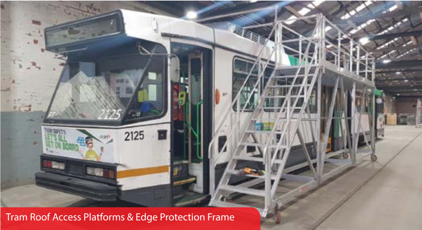
Adjustable Height Cantilever Platform with loop Guardrail; for Train Roof Inspection & Access
