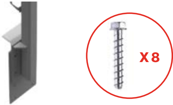
QTY 4: 10 x 60mmL concrete seismic concrete screw anchor QTY 4: 10 x 70mmL concrete seismic concrete screw anchor *50mm embedment
