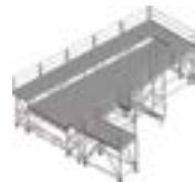
Cargo Door Operating Stand Guardrails slide out to allow access to the door activation handle.
