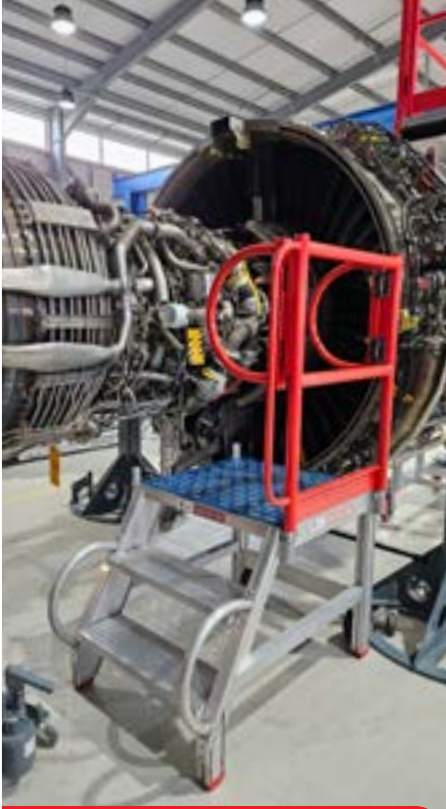
Handles for manoeuvrability, simply lift to engage the front wheels.
